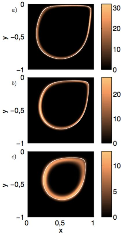
Figure A: Comparison between optimal streamlines of WKBJ eigenmodes (short-wave analysis) and inviscid structural sensitivity maps related to (Global) eigenvalues: a)  $0.36 + i0.00$ ; b)  $0.14 + i0.20$ ; c)  $0.07 + i0.00$ . Parameter settings:  $\text{Re}\{\text{BaseFlow}\}=1370$  (where the considered cavity flow first undergoes a pitchfork 3d bifurcation),  $\text{Re}\{\text{Stability}\}=300000$  &  $k = 93.5$  (spanwise wavenumber).
